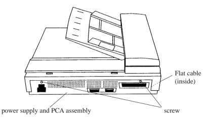
(5) Remove the two screws in the following figure.
